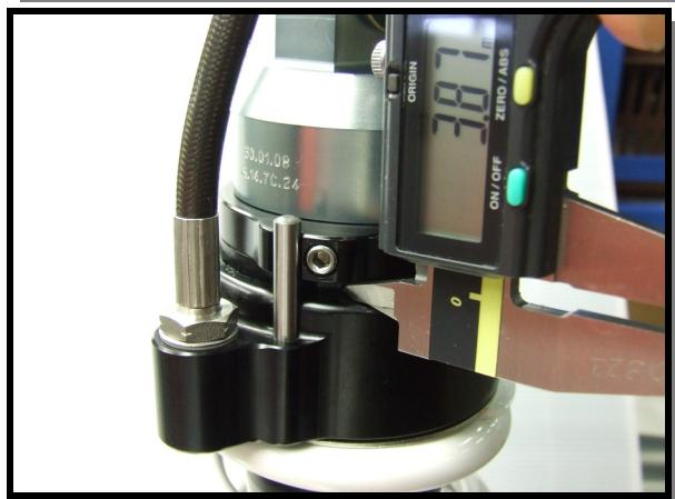
This can be set by counting the revolutions of the knob (see above), or measuring the distance as shown. (more accurate)
