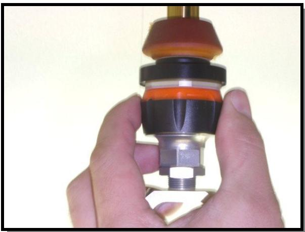
The adjuster on the lower part of the shockabsorber is the rebound adjuster
