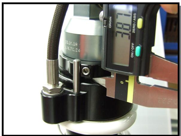
If the damper has a Pre-load adjuster: Mark the position of the adjuster, to be able to set the same amount of Pre-load.
