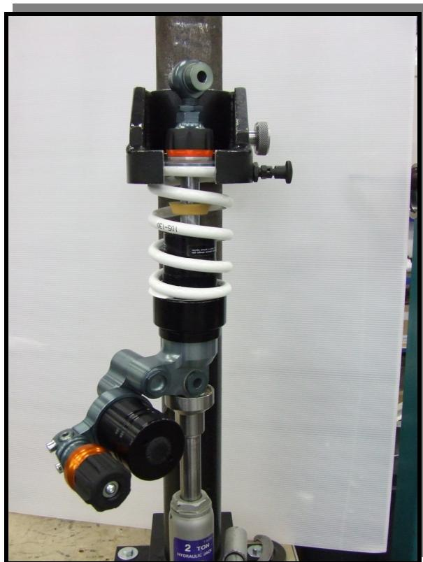
Put the Pre-load adjuster into it's minimum position.
