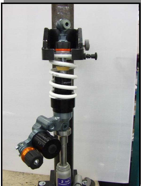
Put the shock absorber in the hydraulic press, or use a spring release tool.
