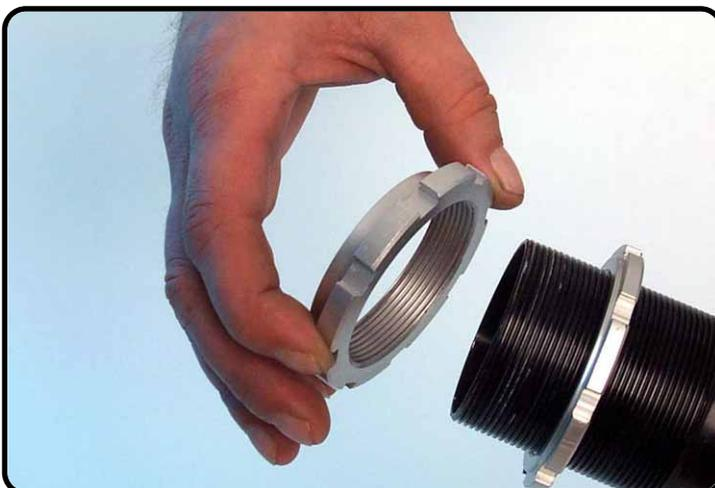
Assemble both spring retainers on threaded bush.
