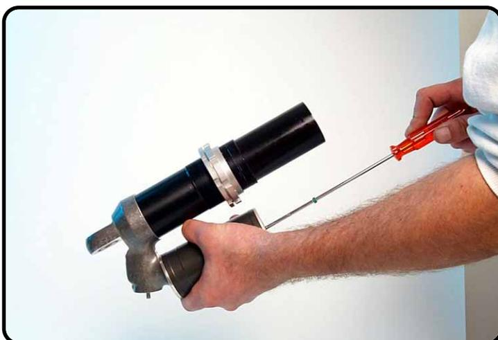
Push the separation piston downwards, and hold the tube side in a angle. (about 45 degrees)
