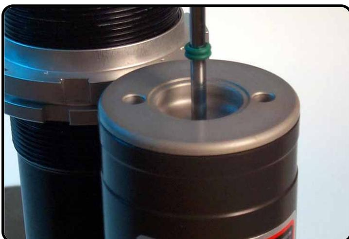
Adjust separation piston about 10mm from the bottom, O-ring on the shaft will be 10mm above the screw-cap.
