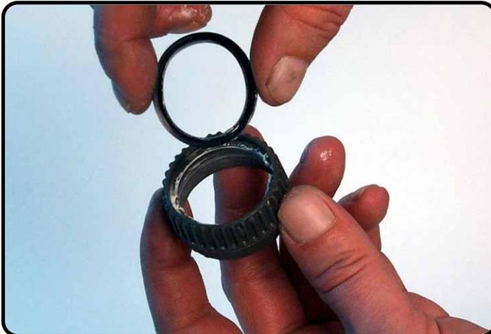
Grease innerside adjusting knob with T159 and replace the seal.
