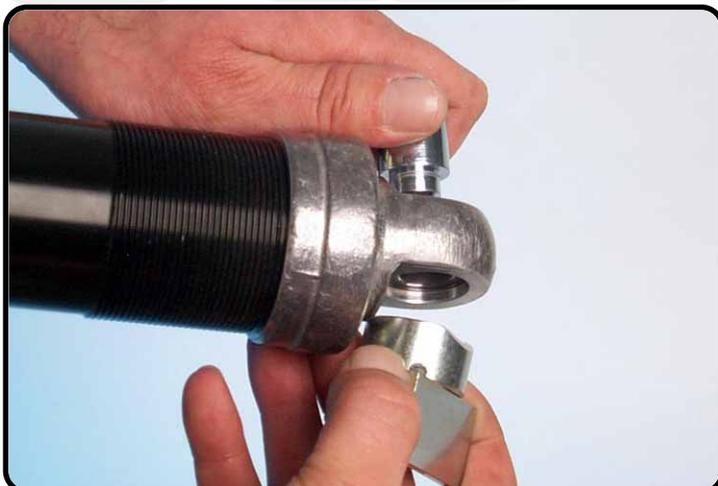
Disassemble the heim-joint KGW with T130S...
