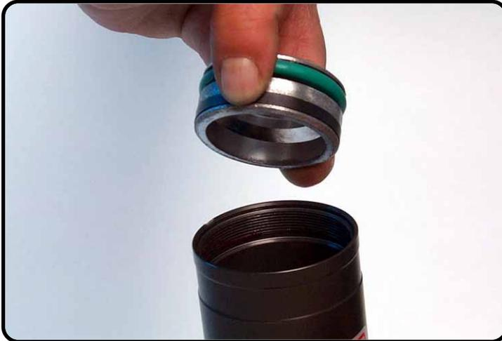
Assemble separation piston (with piston-ring) always into direction of the screw-cap.
