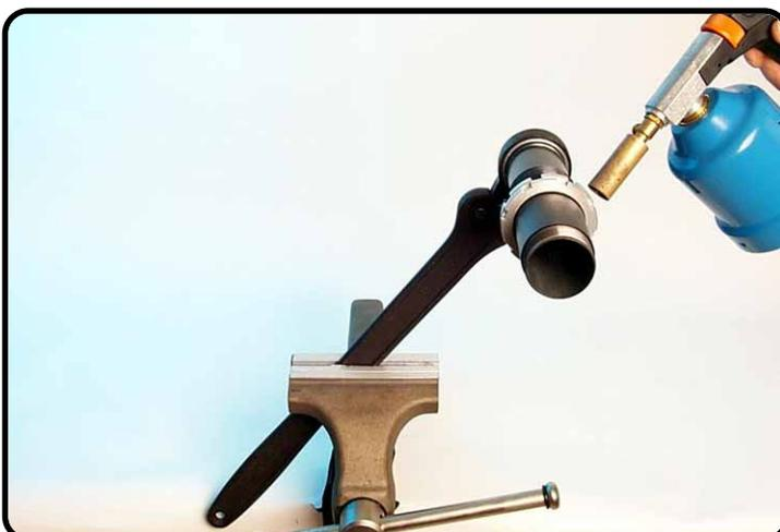
Clamp the tube with T146 and T148 and heat the threaded bush.
