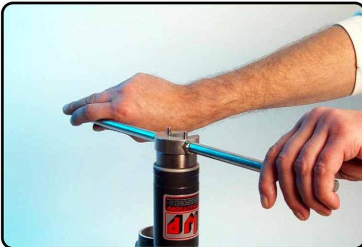
Tighten the screw-cap and reservoir with T125S and T145S.
