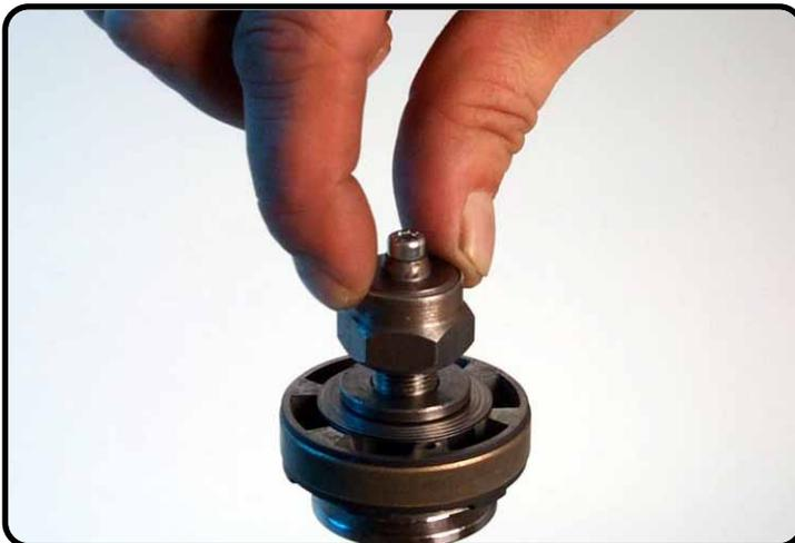
Screw the piston-rod nut on piston-rod....
