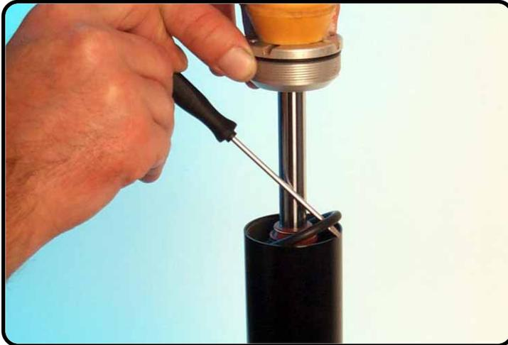
Lift the O-ring out of the tube.
