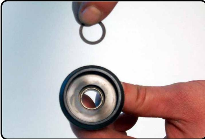
Assemble the back-up ring.
