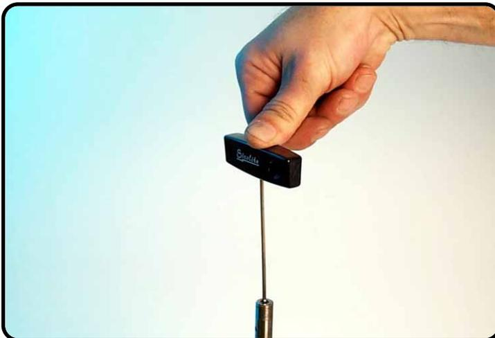
Push needle downwards on pin with Allenkey size 2.
