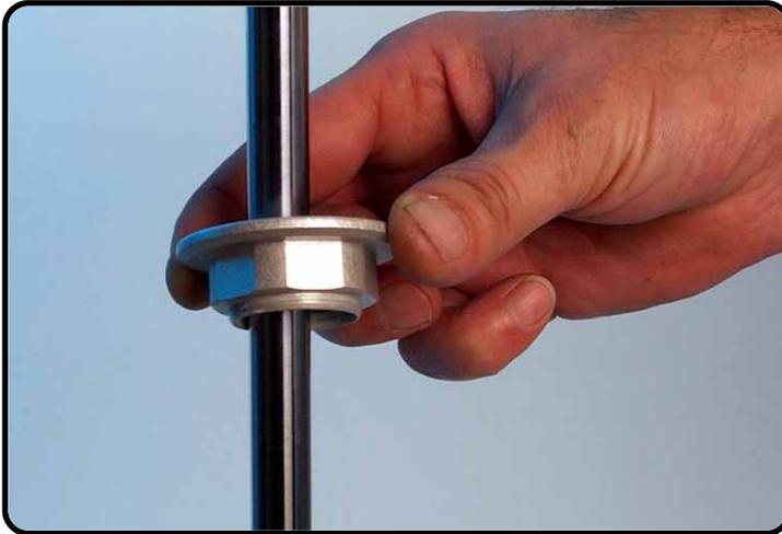
Remove the steel washer and springing.
