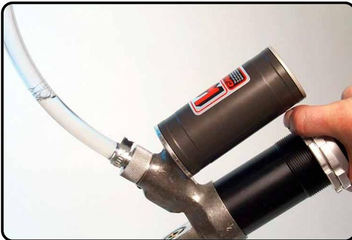
Turn to a view times the shock absorber and repeat the procedures several times until all air is bled out.
