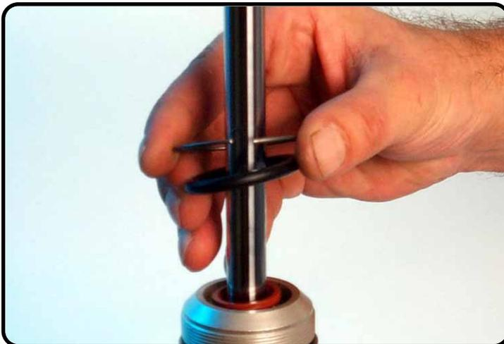
Remove the circlip and O-ring.
