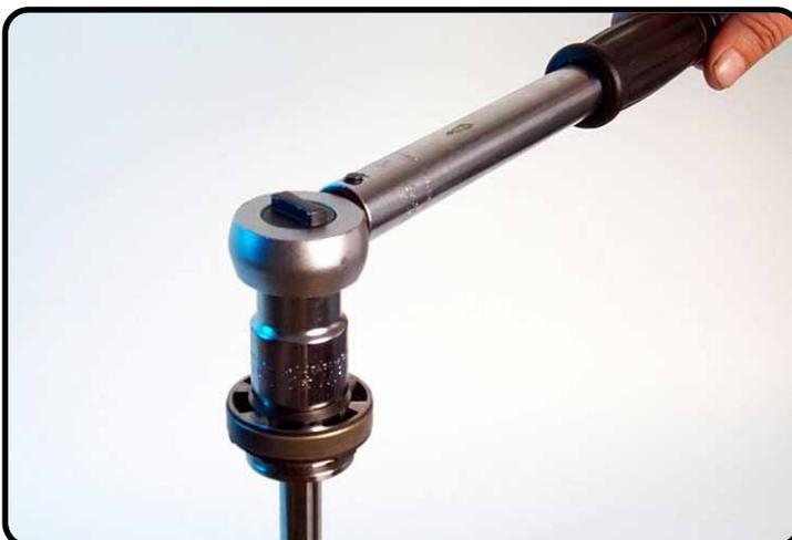
...and tighten the nut to a torque of 40Nm.
