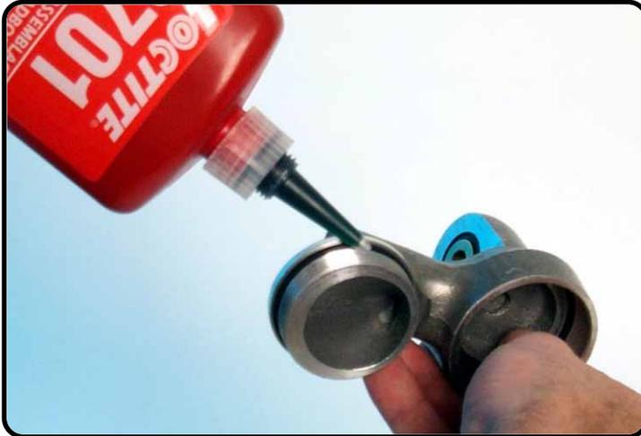
Drip T132 on thread of the bottom.
