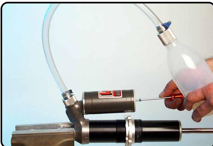
Check the position of the separation piston with T107S.
