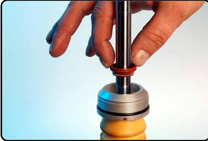
Grease the innerside dirt scraper with T625 and assemble.
