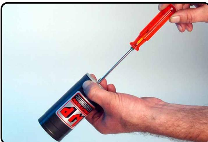
Push the separation piston out of the reservoir with T107S.
