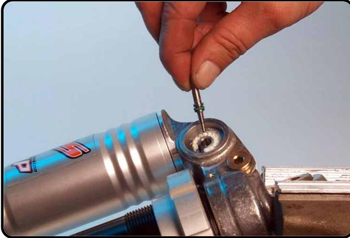
Screw the adjusting needle hand tight into mechanism.
