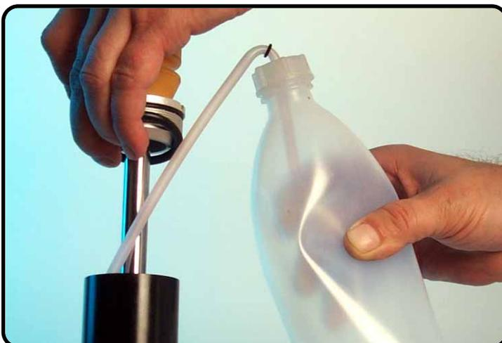
Remove (if necessary) the oil above the adaptor with T137S.
