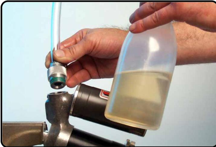
Ensure that there is sufficient oil in the bottle and that the hose is also full with oil. You will see air bubbles rising up through the hose.
