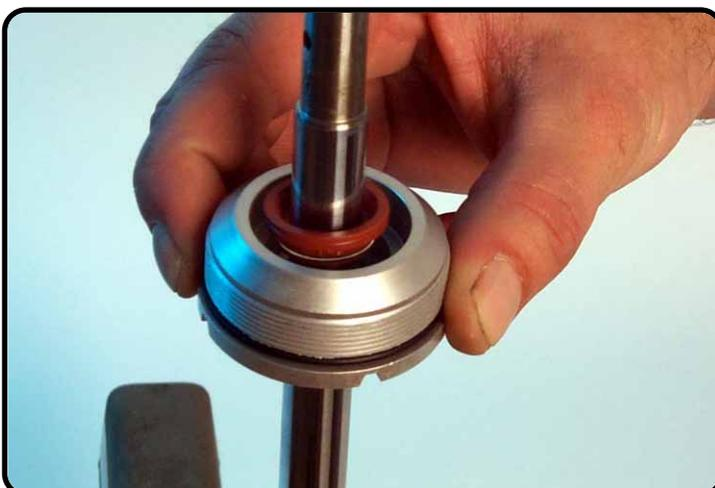
Remove the dirt scraper and screw-cap.
