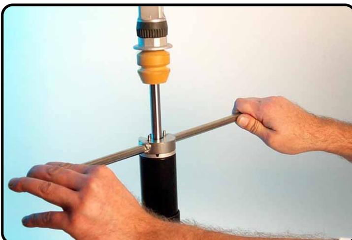
Unscrew the screw-cap with T125S.
