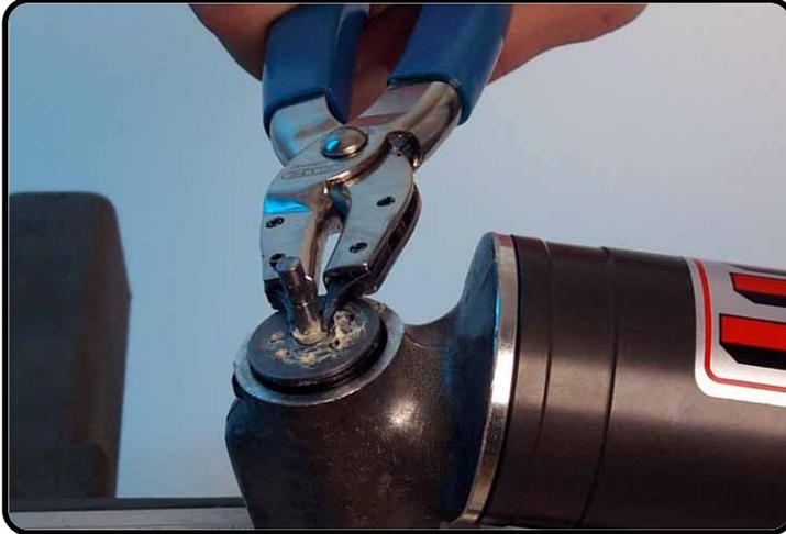
Connect the adaptor of T144S into the housing.
