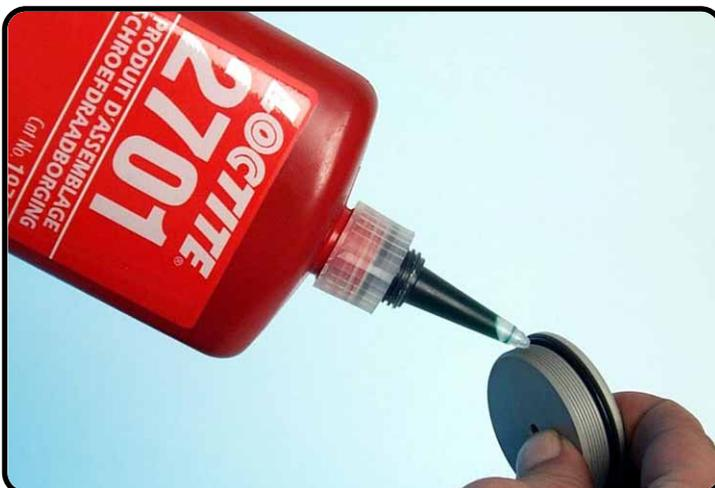
Drip T132 on the thread of the screw-cap.
