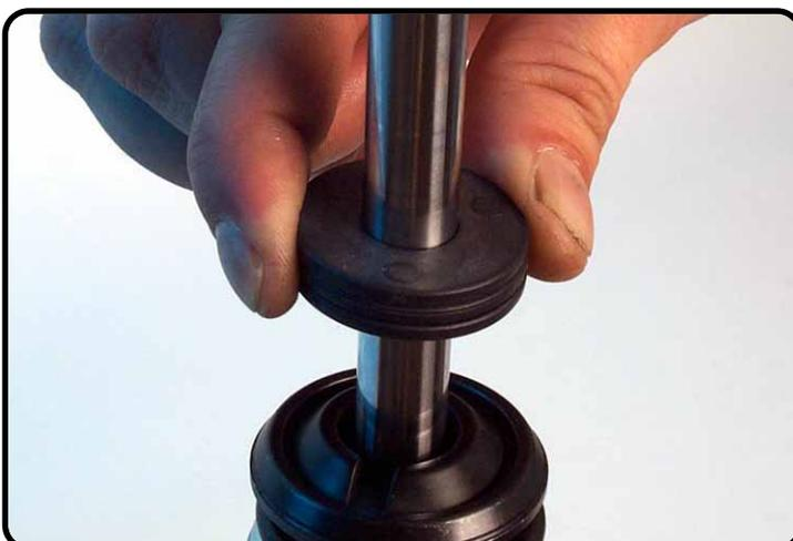
Should it be the case to assemble spacers, then place them with the flat side direction rebound rubber.
