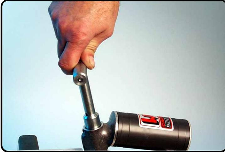
Push the mechanism with T160 past the lock washer groove.
