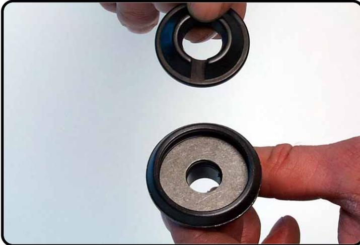
After assembly the rebound rubber, check if the rubber can be rotate in the holder.
