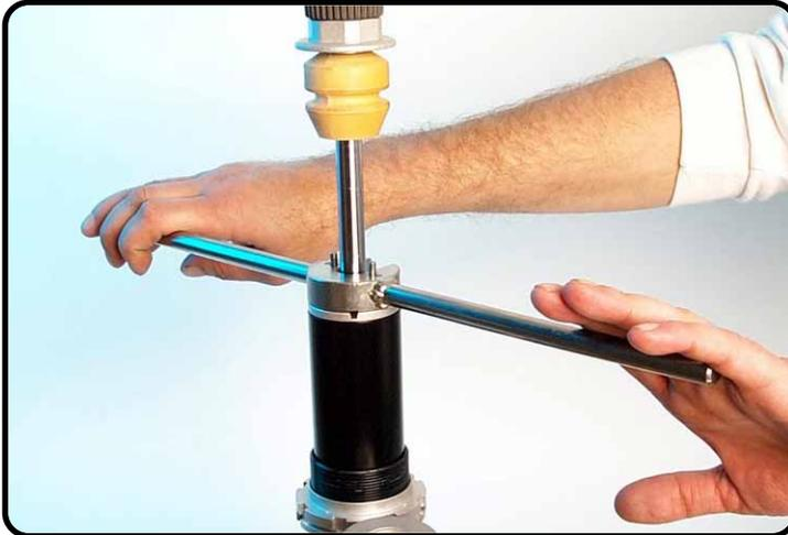
Tighten the screw-cap with T125S.
