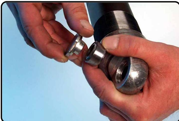
Drip on the innerside of bottom-eye T163 and mount heim-joint KGW with T129. (With the bevelled edge direction bottom-eye)
