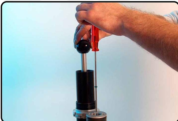
Place T110S in the tube and push the plunger downwards.
