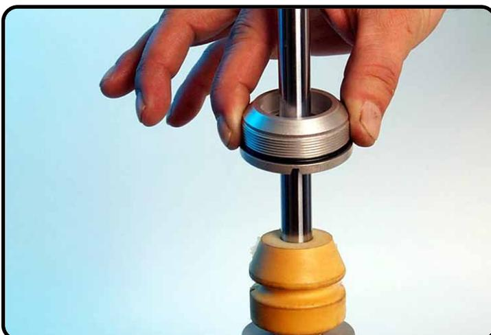
Assemble the screw-cap.
