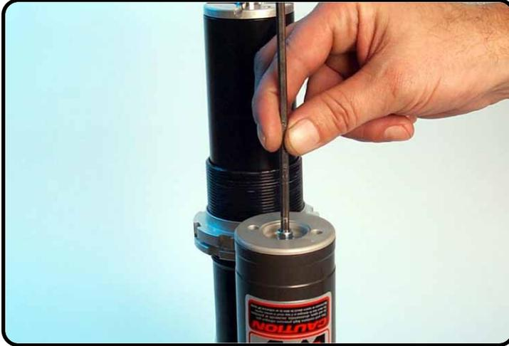
Place the shock absorber (reservoir) in T170S and fill it with nitrogen ( $\pm 20$  sec.) and tighten the plug under pressure.
