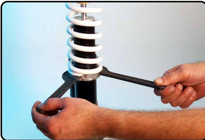
Tighten the spring retainers with T106.
