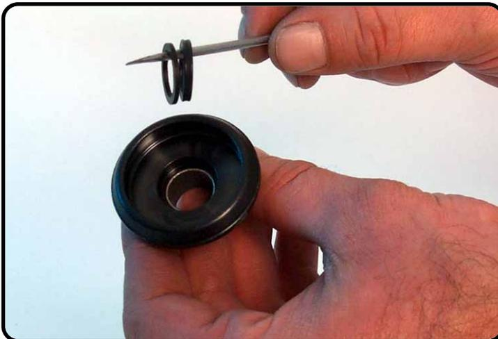
Remove the quad ring and back-up ring.
