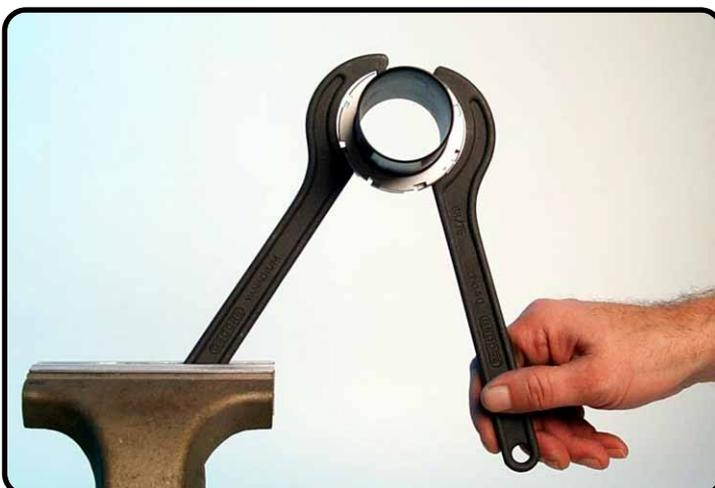
Disassemble the spring retainers with T106.
