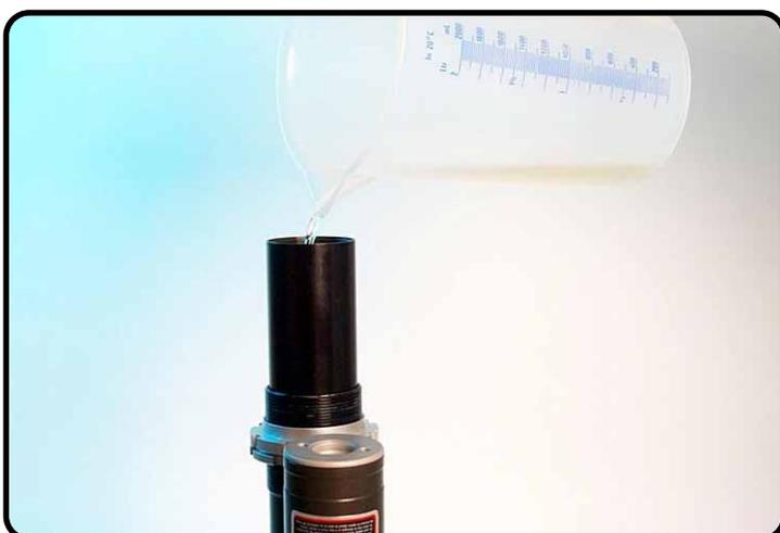
Fill the tube with oil about 15mm under the springing groove.
