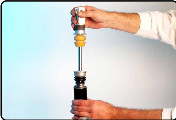
Pull piston-rod "complete" out of the tube.
