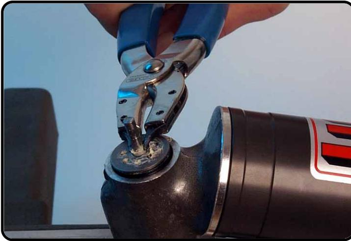
Lift out the compression control mechanism.
