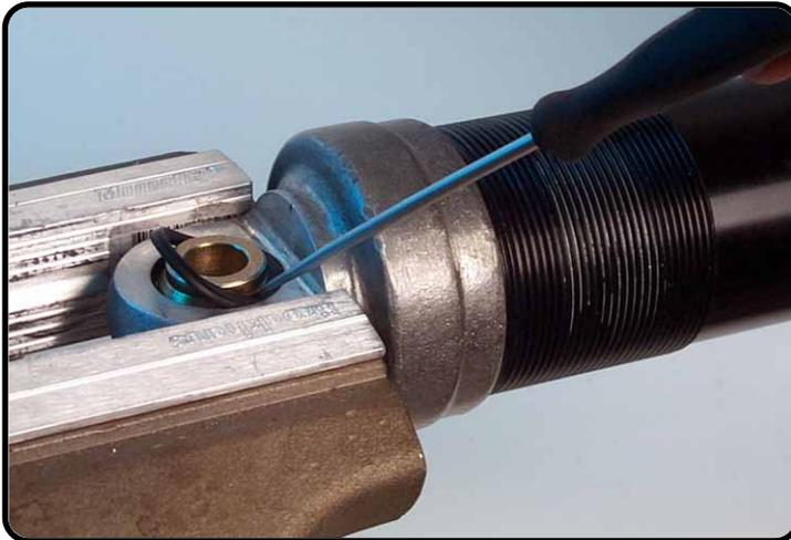
Assemble the seals in the groove of the bottom- eye.
