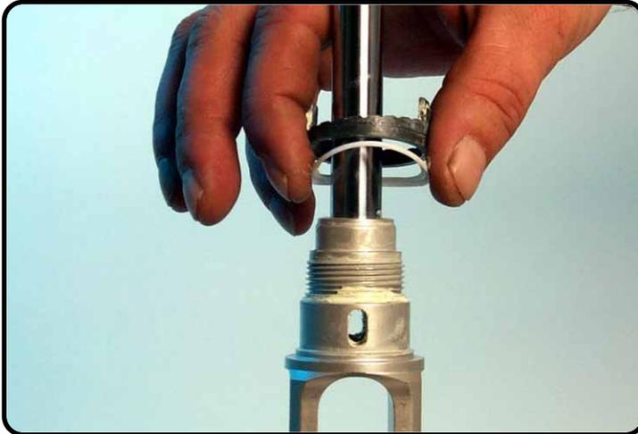
Replace the seal and the position ring.
