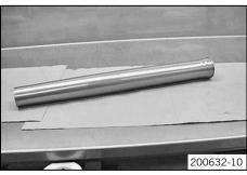
Measure the outside diameter at multiple locations of the inner tube. \_
