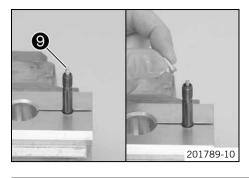
Remove valve needle 9 from the piston rod.
