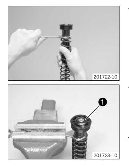
Pull the spring down. Mount the open end wrench on the hexagonal part.
