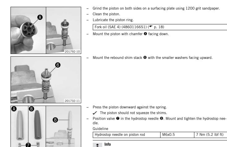
silver hydrostop needle on compression damping side.
