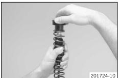
Clamp the open end wrench in the vise. Release screw cap lambda but do not remove it yet.
