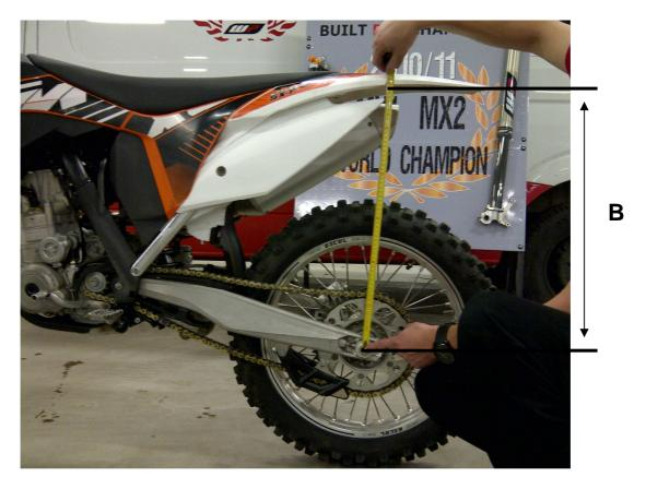
The static sag is the difference between dimension A and B. The static sag should be as close as possible to 35mm. If the sag is lower than 35mm the spring preload must be reduced, and if the static sag is to high the spring preload must be increased.
