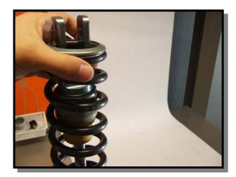
Remove the circlip, spring retainer and washer to be able to take the spring off.
