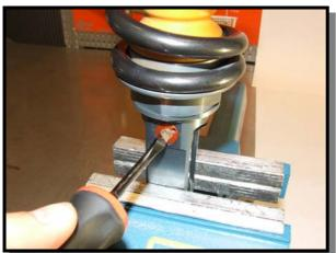
Use a large screwdriver to adjust the rebound damping.
