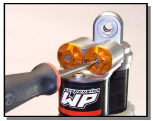
Use a large screwdriver to adjust the compression.
