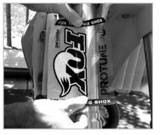
6 Working from the center, press the decal onto the upper tube. Remove the release paper as you apply. Avoid trapping any air bubbles under the decal as you go.
