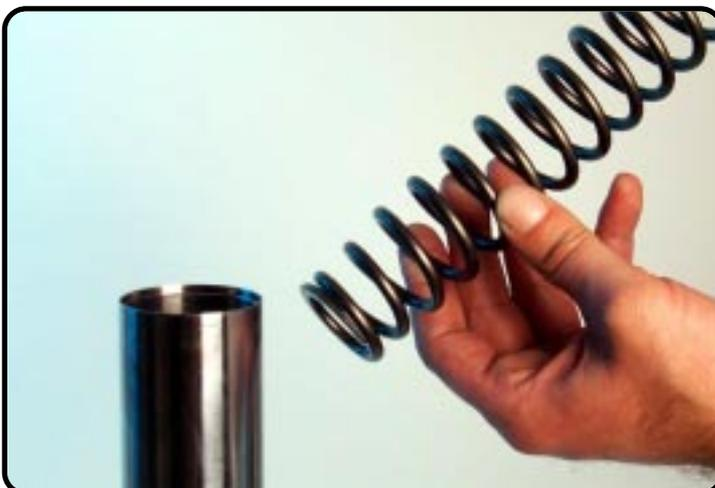
Replace the spring with the conical side under.
