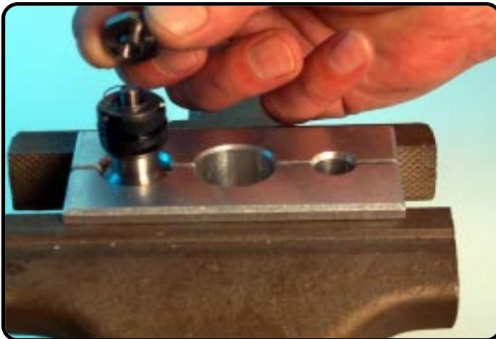
Remove the check-valve nut.
