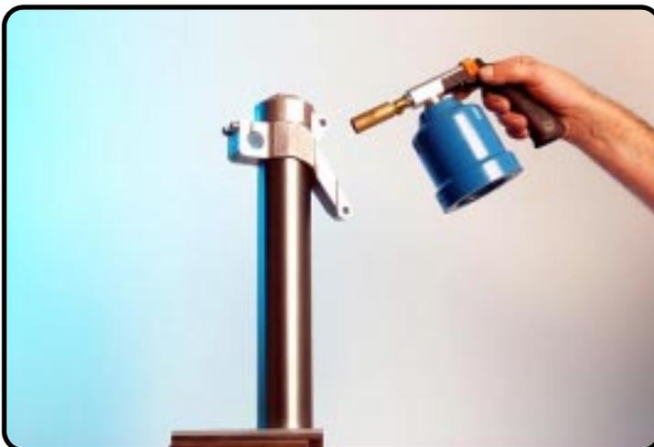
Clamp the outer-tube in the vice and heat the axle-clamp.
