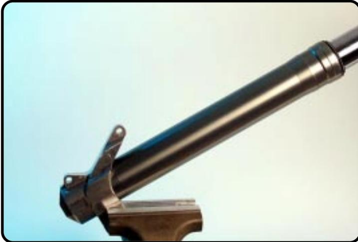
Clamp the axle-clamp in the vice so that the forkleg is about a 45 degrees angle.
