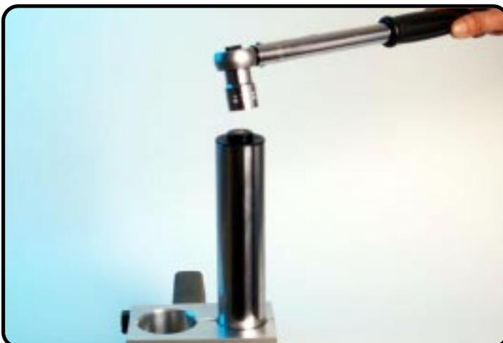
And tighten the screw-cap to a torque of 25Nm.
