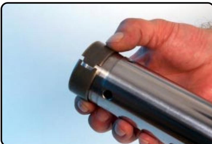
Disassemble the DU-bush of the inner-tube.
