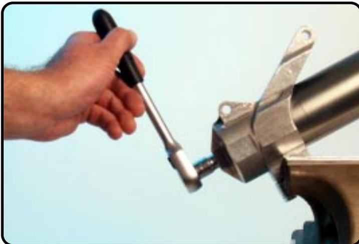
Unscrew the bolt out of the axle-clamp.
