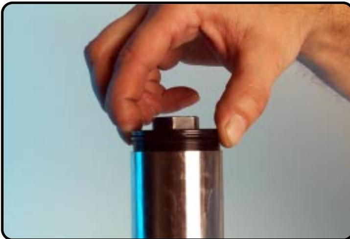
Screw the screw-cap into the inner-tube.
