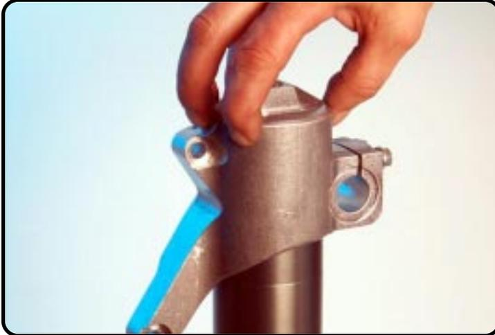
Clamp the outer-tube with T904S inside in the clamping block and assemble the axle-clamp.
