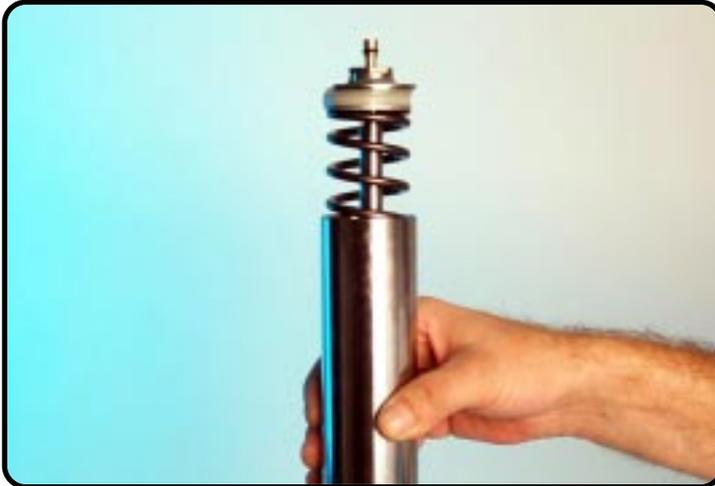
Let the inner-tube down into the outer-tube.
