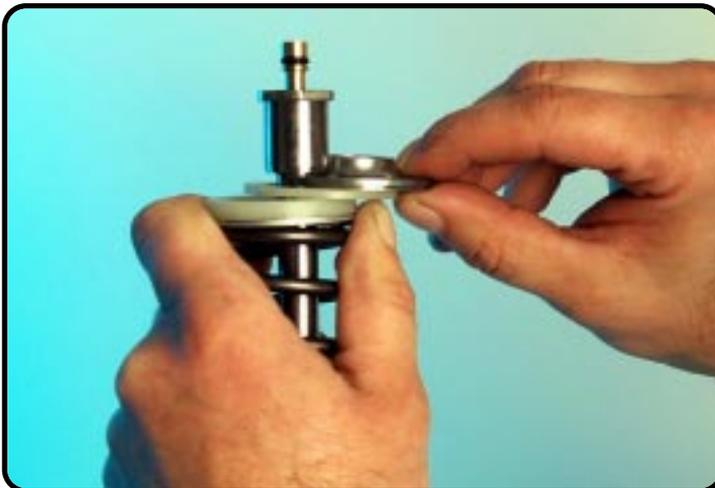
Remove the spring retainer, preload spacers and steel washer.
