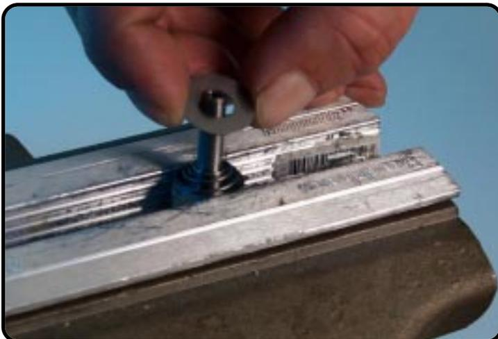
Disassemble the shim for check-valve.
