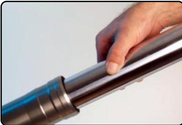
Slide the inner-tube slowly in the outer-tube.
