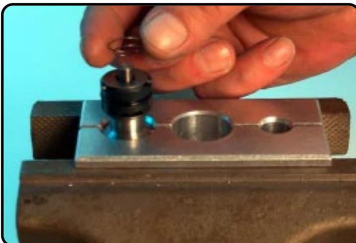
Remove the spring for check-valve.
