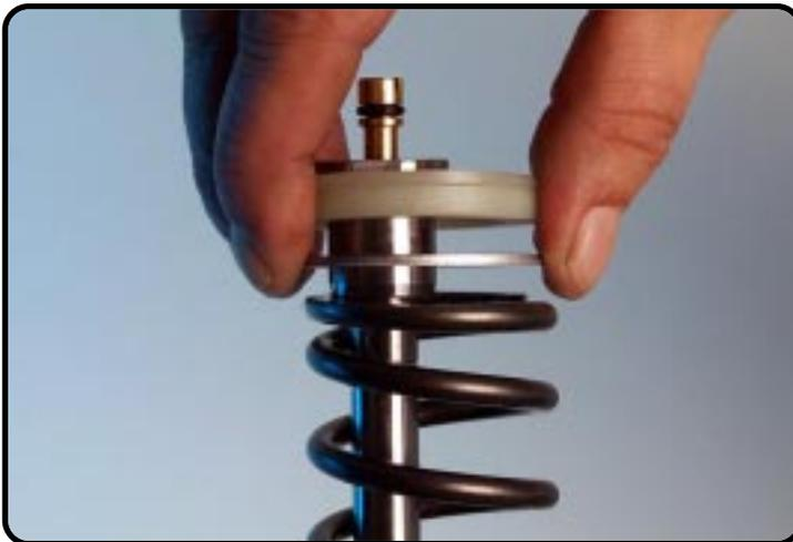
Replace the steel washer and the preload spacers.
