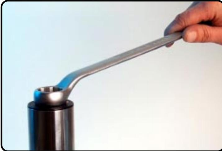
Disassemble the screw-cap.
