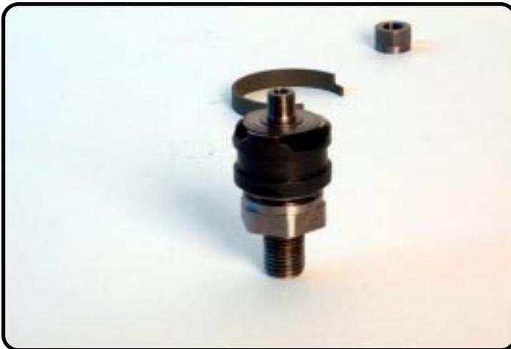
Assemble the shim for checke-valve, piston and rebound shims.
