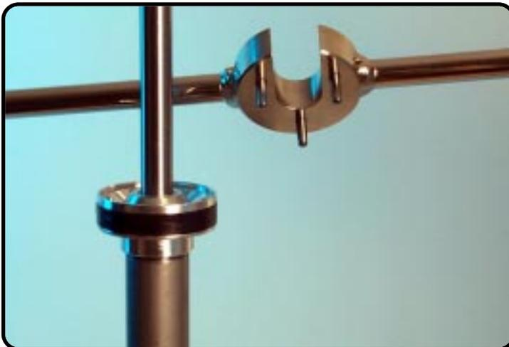
Assemble T907S on the screw-cap.
