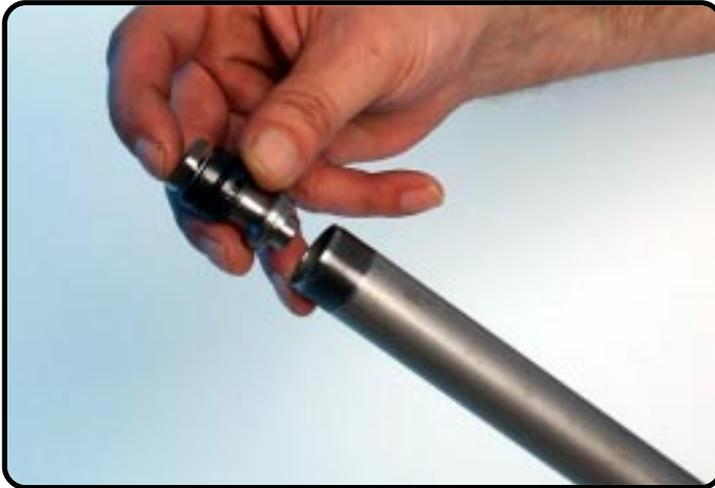
Assemble the tap compression into the tube.
