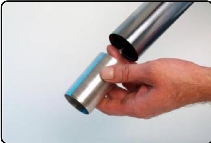
Hold forkleg up side down and remove the house hydraulic stop.
