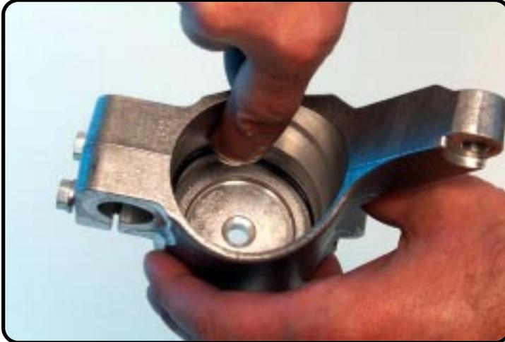
Wetting the thread of the inner-tube with T132.
