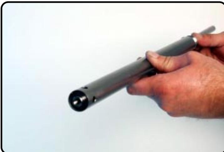
Push with support of the piston-rod the tap compression till the springing.
