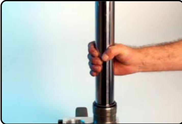
Moving the inner-tube 'not too high', up and down.
