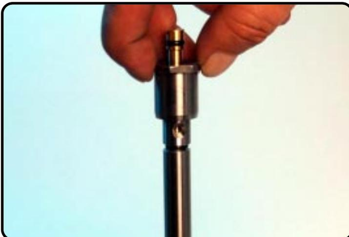
Clamp the piston-rod in on the other side and screw in the piston-rod adaptor.
