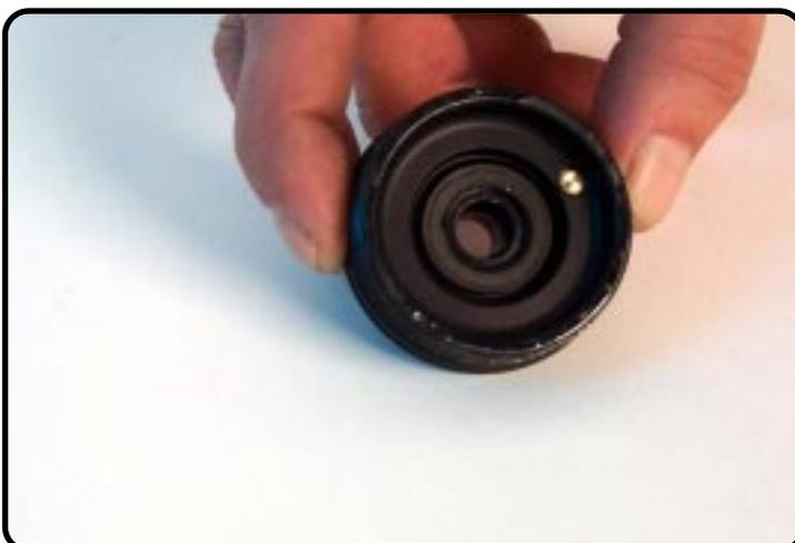
Check the rubber sealing ring inside.
