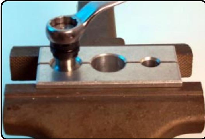
Unscrew the check-valve nut (size 17).
