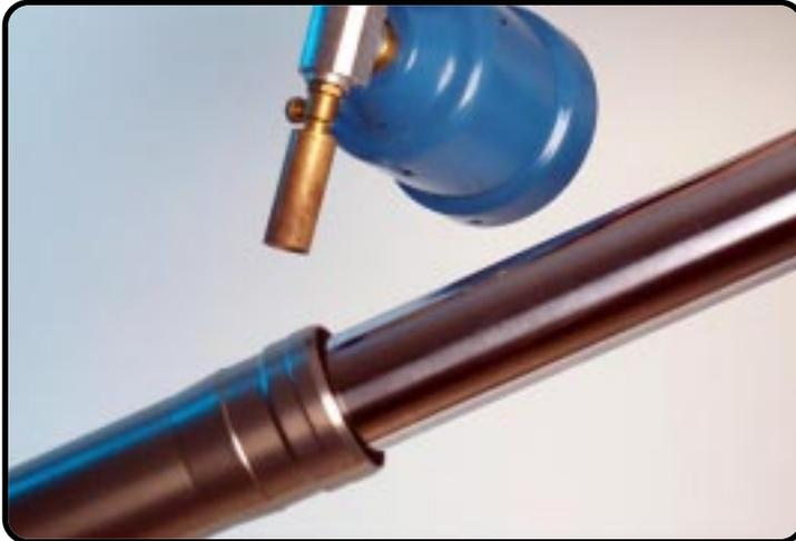
Heat the outer-tube near the oilseal.
