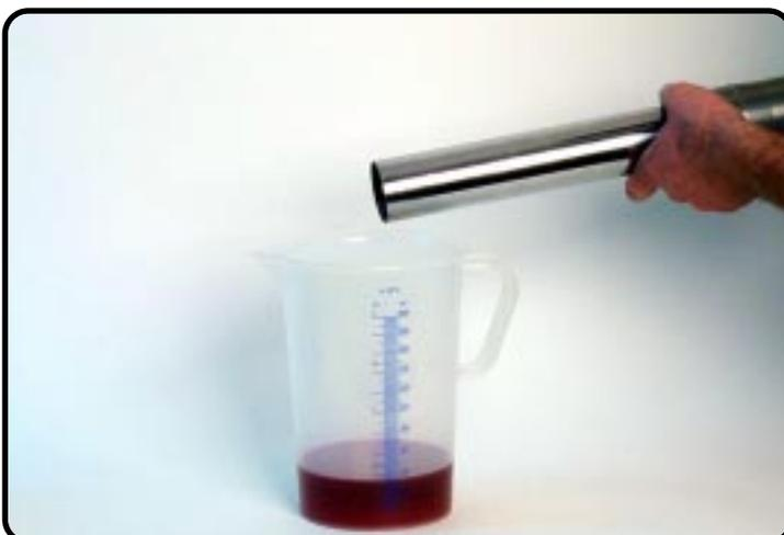
Drain the oil out the forkleg.
