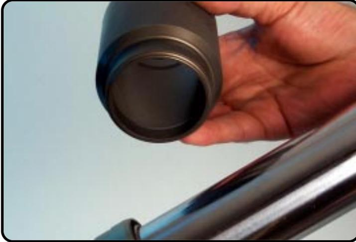
Use T902 -flat side- to tap or push the DU-bush in the outer-tube
