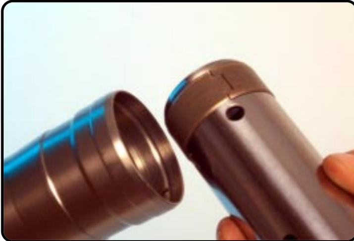
Assemble the DU-bush on the inner-tube and clamp the (axle-clamp) outer-tube in the vice.
