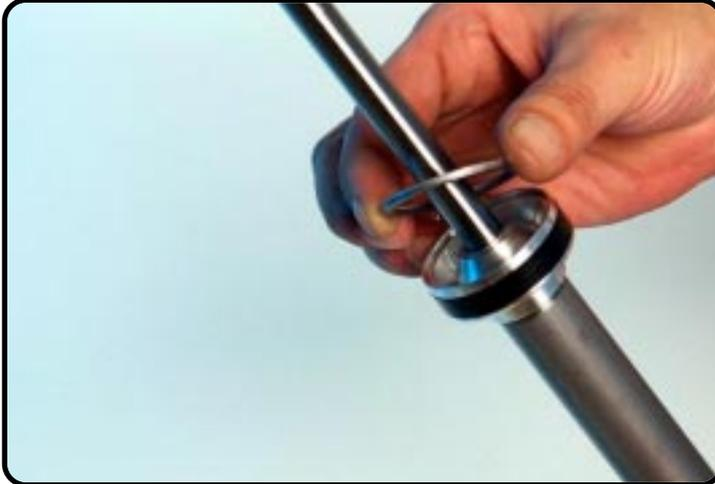
Remove the steel washer.
