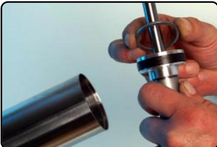
Replace the steel washer. Pay attention to the assembling direction!!!
