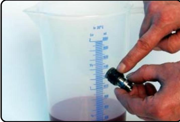
Grease the O-ring of the piston with frontfork oil.
