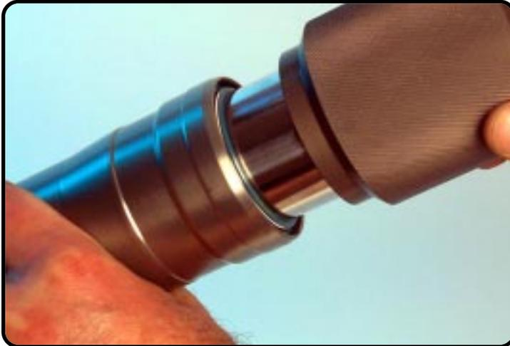
Assemble the oilseal with the other side of T902 into the outer-tube.
