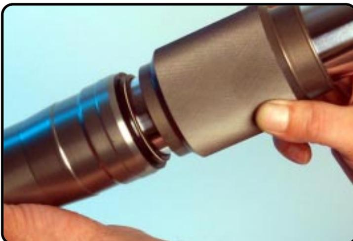
Tapping the dust wiper into the outer-tube.
