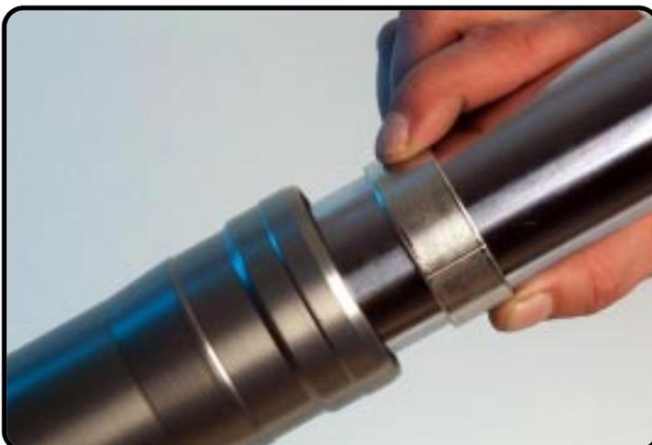
Assemble the DU-bush outer-tube.
