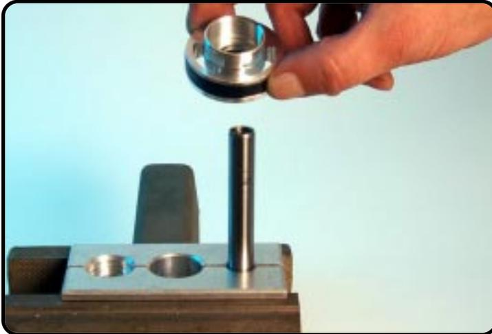
Remove the screw-cap.
