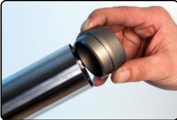
Place T901 on top into the inner-tube.
