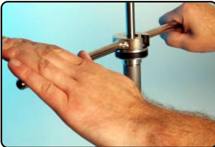
Tighten the screw-cap.
