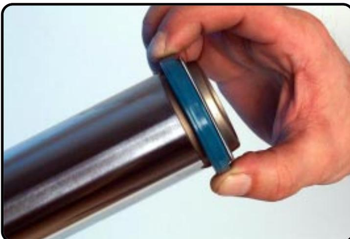
Slide the oilseal over the inner-tube.
