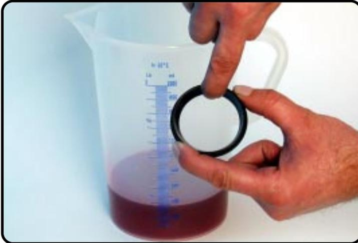
Grease the innerside of the dust wiper with frontfork oil.
