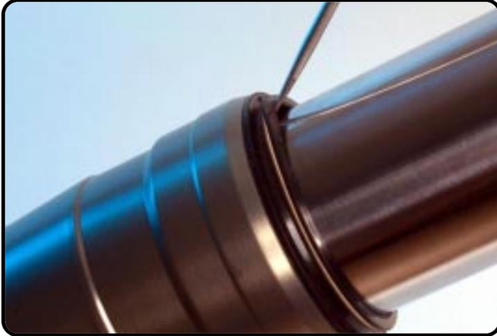
Release carefully the air between the assembled dust wiper and outer-tube with a small screwdriver.
