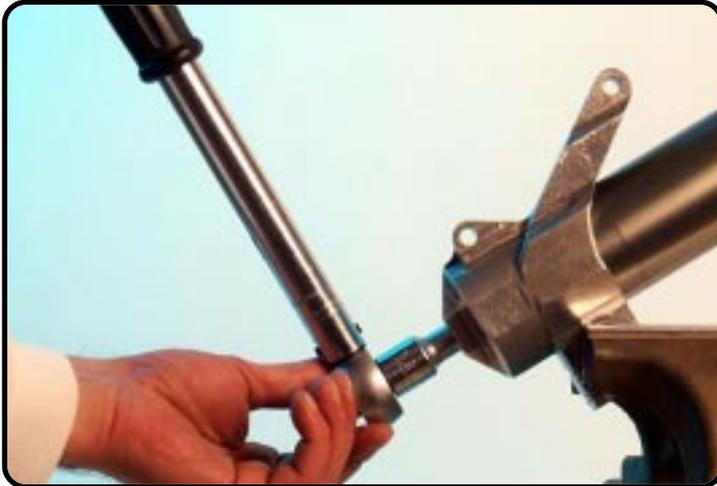
Tighten the bolt to a torque of 22Nm.
