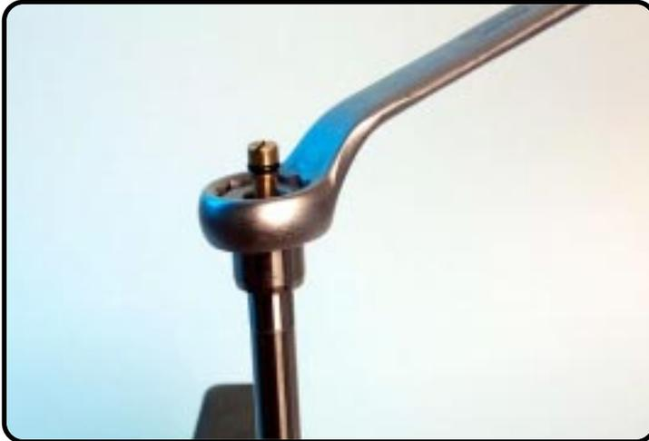
Tighten the piston-rod adaptor.
