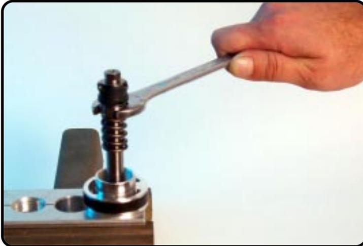
Unscrew the rod tap from the piston-rod.
