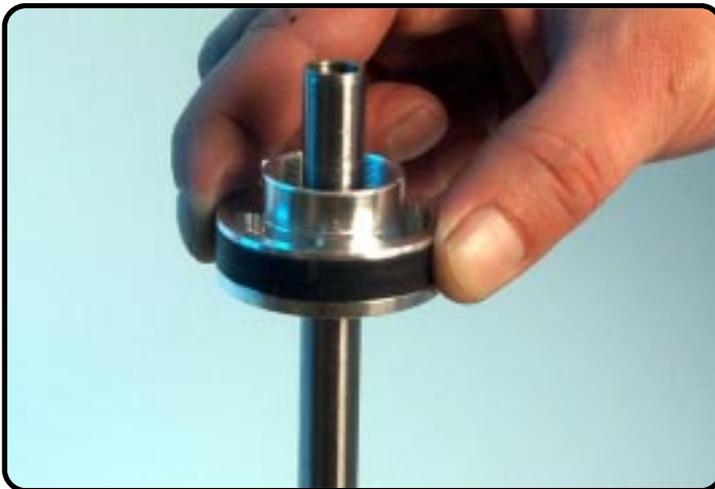
Assemble the screw-cap with steel washer.
