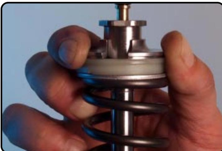
Assemble the spring retainer
