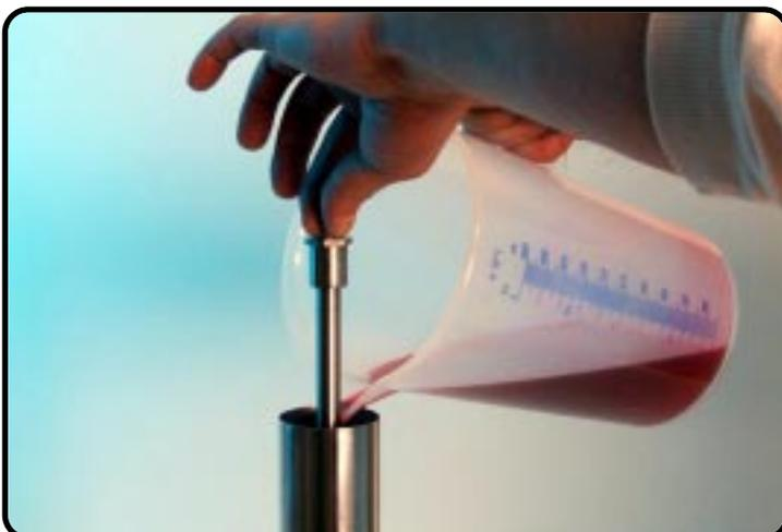
Fill the forkleg with oil just under the edge of the fully compressed inner-tube.
