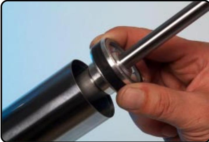
Assemble the cartridge into the forkleg.
