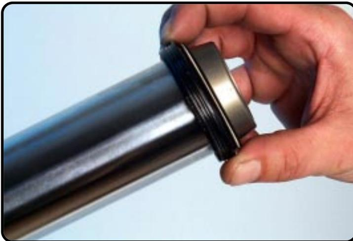
Slide the dust wiper on the inner-tube.
