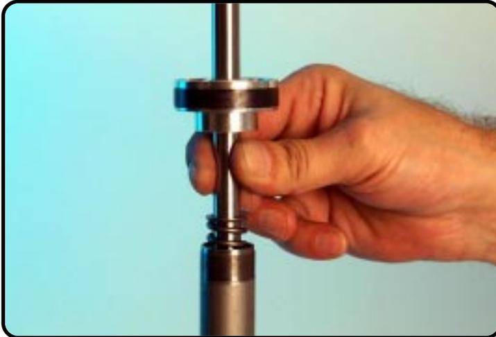
Pull the piston-rod out of the tube.
