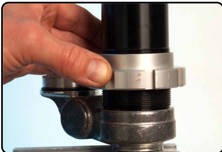
Screw spring retainer from the tube.
