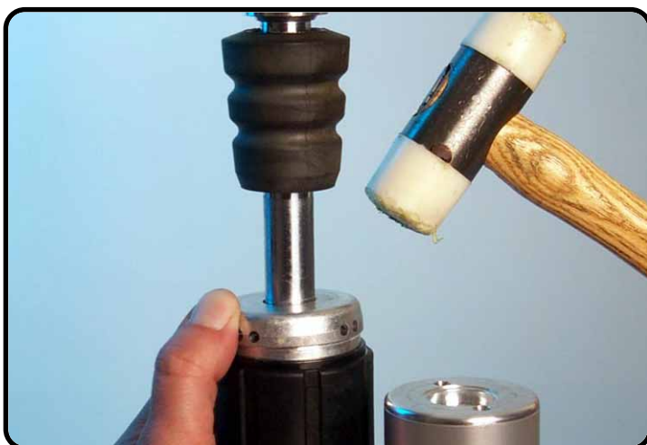
Tap the cap back into position.
