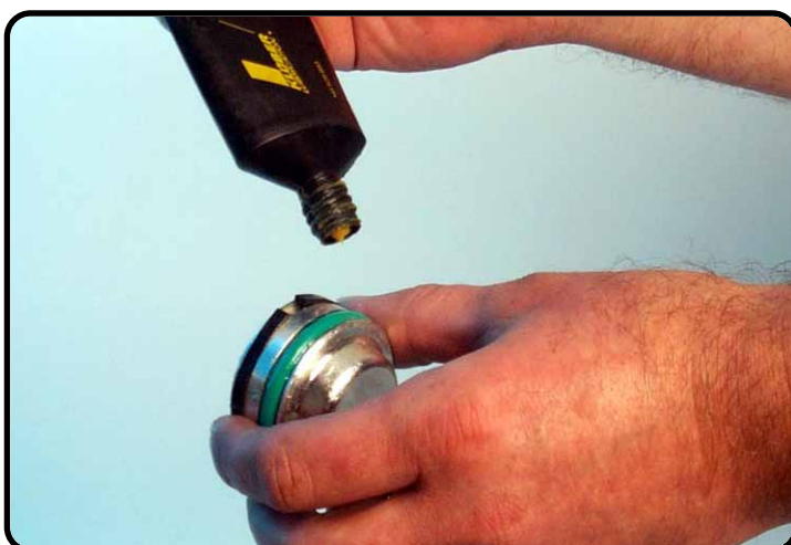
Building up the nitrogen reservoir. Grease the O-ring of the separate piston with T158.
