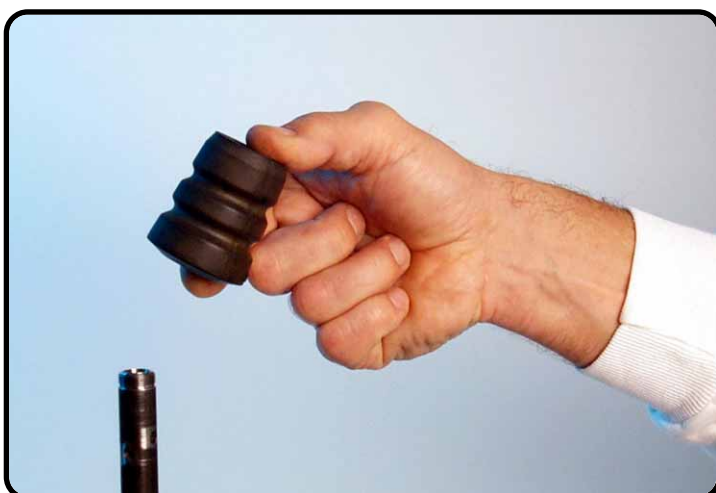
Remove the bump rubber.
