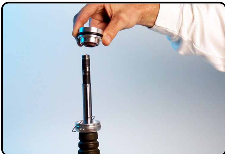
Remove the adaptor DU-bush.
