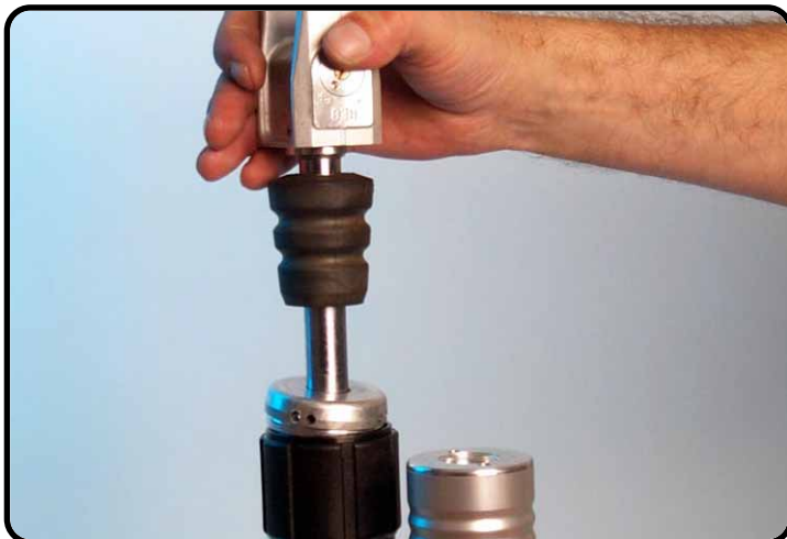
Pull up the piston-rod.
