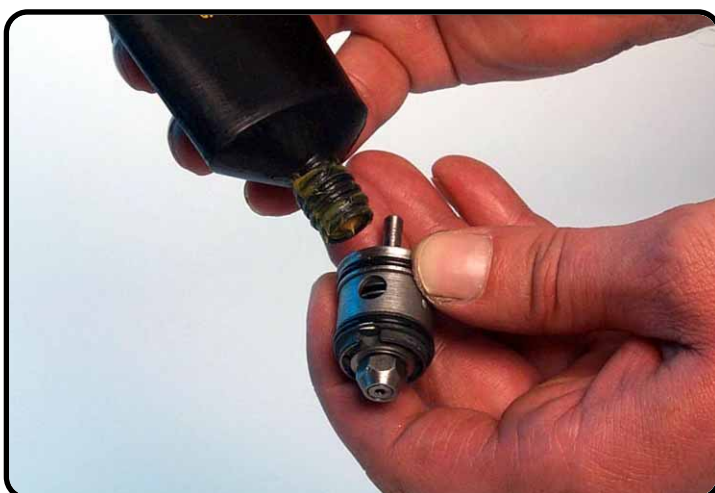
Assembling compression control mechanism. Grease the O-rings with T158.
