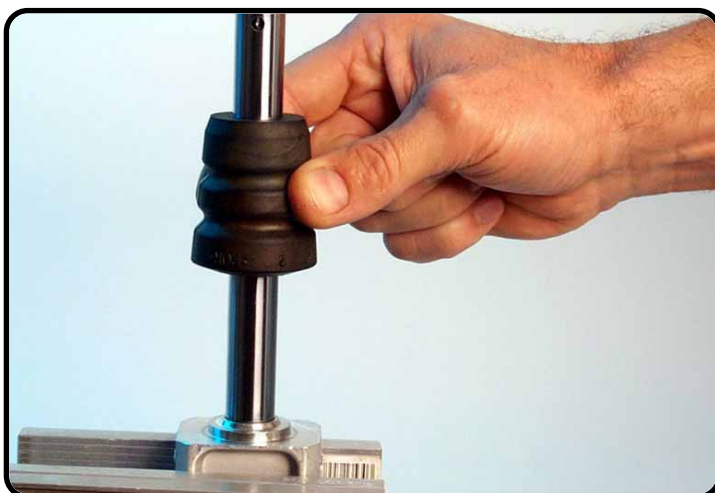
Assemble the bump rubber.
