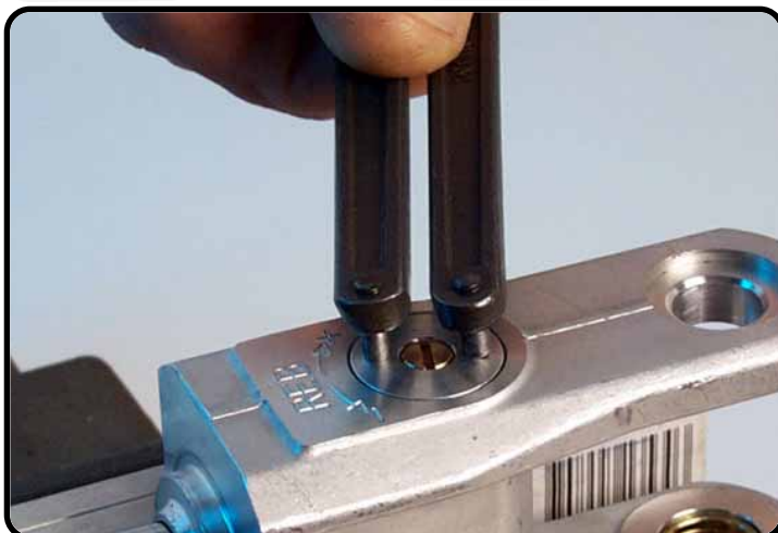
Disassemble screw-cap rebound damping holder with T1218.
